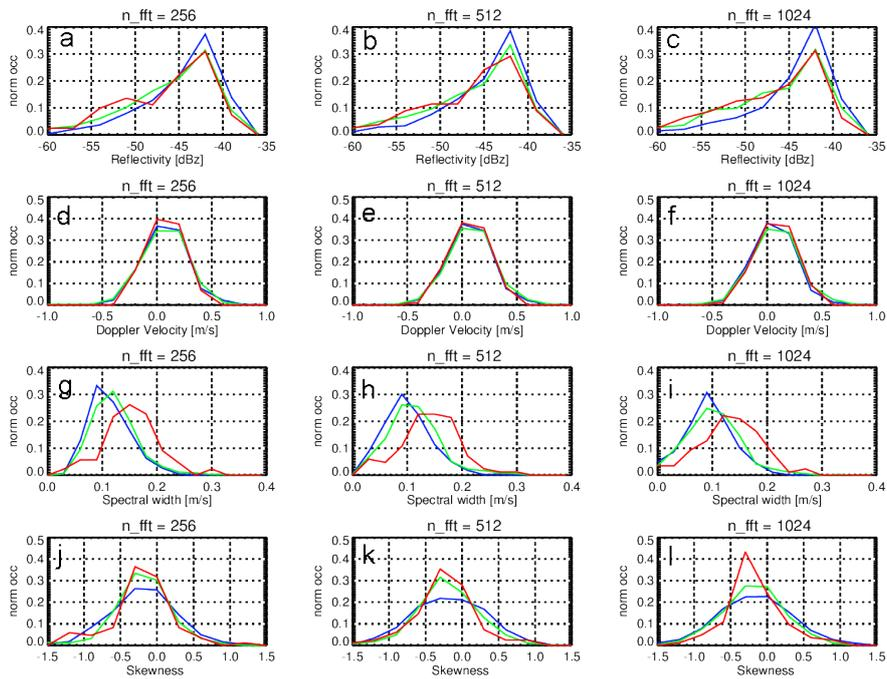
Figure S 1 – Distributions of moments for the case of the 20 November 2014. Each line of the figure shows the distribution for a given moment at the different fft lengths (from left to right 256, 512 and 1024): reflectivity ( $Z_e$ ) on the first line, mean Doppler velocity ( $V_d$ ) on the second line, Spectral Width ( $S_w$ ) on the third line, Skewness ( $S_k$ ) on the fourth line. Different colors correspond to different integration times: red (10 s), green (2 s) and blue (0.4 s).
