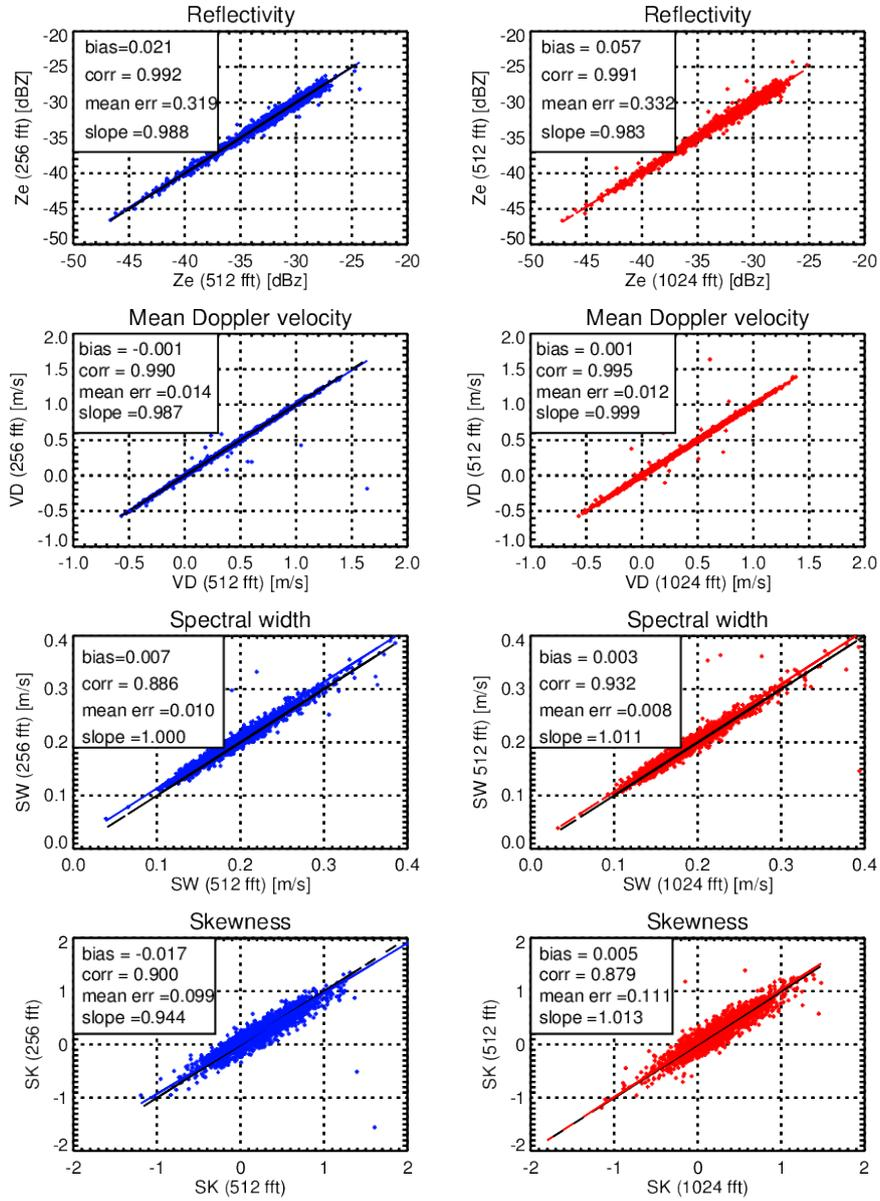
Figure S 3 – Effect of spectra resolution on moments: scatter plot of moments derived at 256 ft length with the corresponding ones derived using 512 ft length for the case of the 24 June 2015. All the spectra are calculated with 2 s integration time. The left column compares 512 with 256, while the right column compares the 1024 ft length with the 512 ft length.
