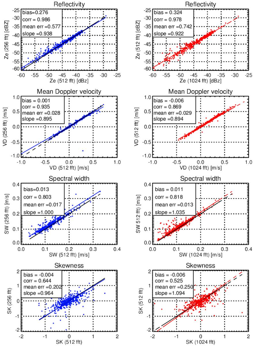
Figure S 2 – Effect of spectra resolution on moments: scatter plot of moments derived at 256 ft length with the corresponding ones derived using 512 ft length for the case of the 20 November 2014. All the spectra are calculated with 2 s integration time. The left column compares 512 with 256, while the right column compares the 1024 ft length with the 512 ft length.
