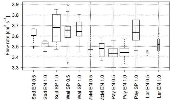
**Figure 2.** Ozonesonde pump flow rates ( $\text{cm}^3 \text{s}^{-1}$ ) measured at the different stations, following the nomenclature of Fig. 1 for the station and ozonesonde.
