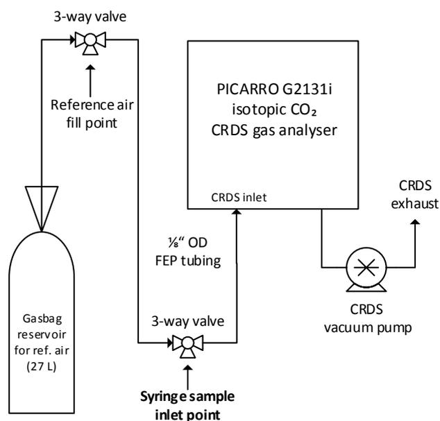
**Figure 1.** Schematic diagram of the discrete gas sample measurement system coupled to the isotopic-CO<sub>2</sub> CRDS analyser.
