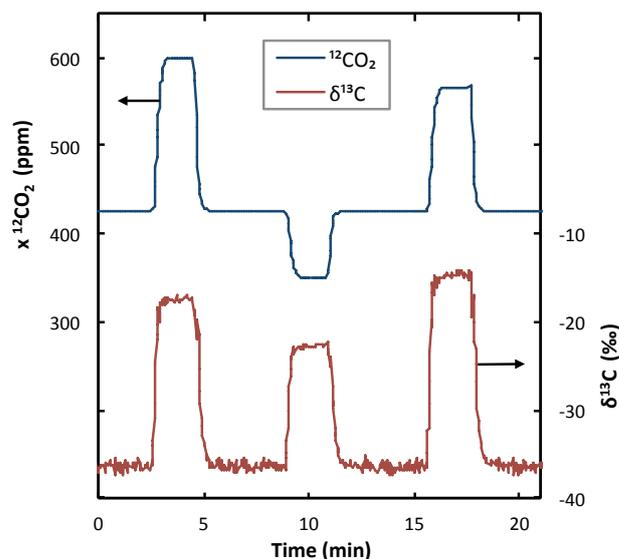
**Figure 2.** Example CRDS data feed for syringe samples. Reference air measurements (ca. 425 ppm  $x^{12}\text{CO}_2$  and  $-37$  ‰  $\delta^{13}\text{C}\text{-CO}_2$ ) are interrupted by successive samples to form consistently identifiable peaks in the data.
