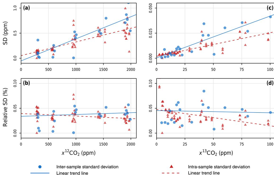
**Figure 5.** Precision in syringe sample data for  $x^{12}\text{CO}_2$  (a, b) and  $x^{13}\text{CO}_2$  (c, d) as quantified by standard deviations (a, c) and relative standard deviations (b, d) for individual measurements (red) and replicate measurements (blue).
