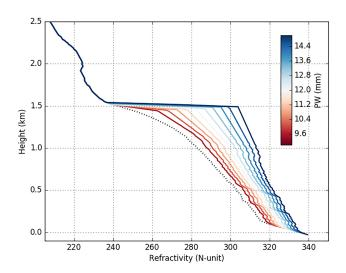
**Figure 2.** The family of refractivity profiles calculated from a single simulated GNSS-RO bending angle profile (dotted line) using Eq. (9) and the parameterization method described in Sect. 2.2.1. Each profile corresponds to a distinctive PW value, which can be used as a constraint for GNSS-RO retrievals within the boundary layer.
