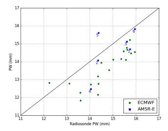
**Figure 8.** PW scatter plot for simulation results from different sources. All 19 RAOB cases PW are compared with the collocated ECMWF and AMSR-E PW in this figure. The *x* axis is the RAOB PW, and the black line is the identity line. ECMWF PW values are systematically lower (1 to 2 mm) than RAOB PW and cause negative biases in reconstructed profiles.
