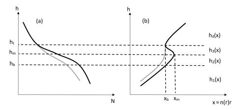
**Figure 1.** The illustration of the corresponding refractivity profile (a) and the h(x) function (b) when ducting occurs. The true profiles are shown in black and the profiles acquired by GNSS-RO Abel retrievals are shown in grey. The large refractivity gradient between  $h_{\rm m}$  and  $h_{\rm t}$  causes the negative slope of  $h_3(x)$  and the multivalued function h(x) between  $x_{\rm b}$  and  $x_{\rm m}$ .
