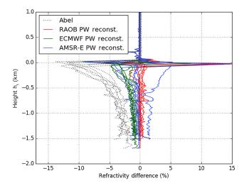
**Figure 7.** Refractivity differences of the Abel-retrieved and the reconstructed profiles from different PW sources compared to the original RAOB profiles in the six simulated cases. It can be seen that the results using ECMWF PW are negatively biased (-1 to -5%) while the collocated AMSR-E reconstructed results more closely aligned with the RAOB profiles. An outlier of the AMSR-E reconstruction shown in the figure is case 5, which was measured 431 km away from the corresponding RAOB case.
