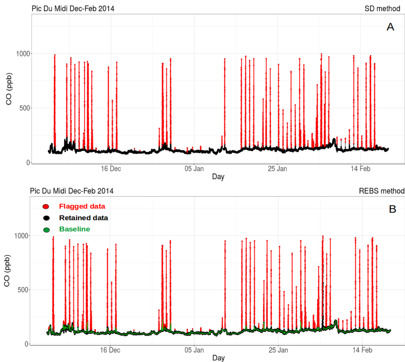
Figure S6: CO measurements from December to February 2014 at Pic Du Midi. Black (red) data points are the retained (flagged) measurements detected by SD method (A), and REBS method (B). The contaminated data linked to the snow removal are characterized by very high CO concentrations up to 1000 ppb.
