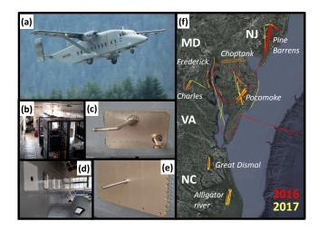
**Figure 1.** The CARAFE payload. (a) The NASA C-23B Sherpa. (b) A view inside the cabin with all instruments installed. (c) The angle-of-attack (upper) and total air temperature (lower) probes. (d) The DLH window plate (upper left) and fairing-mounted target (lower right). (e) GHG inlet. (f) Flux leg flight tracks for both campaigns. Target locations indicated in italicized text correspond to those listed in Supplement Table S1.
