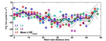
**Figure 11.** Comparison of horizontal CO<sub>2</sub> flux profiles sampled over the same region of mixed cropland and forest on 4 May 2017. Colored circles represent 2 km average fluxes from each of five consecutive legs. The solid black line, shading, and dotted lines are the mean,  $1\sigma$  random error, and  $2\sigma$  random error, respectively.
