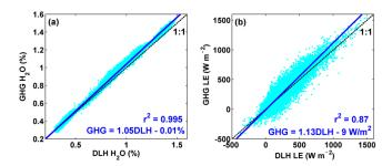
**Figure 10.** Comparison of water vapor mixing ratios (a) and latent heat fluxes (b) for all legs of the 2017 mission. Cyan dots represent 1 Hz average data. Blue lines are reduced major axis linear fits.
