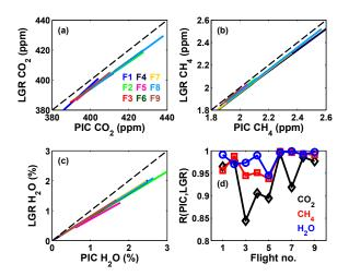
**Figure 2.** Least-squares fit lines (**a–c**) and correlation coefficients (**d**) for Picarro and LGR dry mixing ratios of CO<sub>2</sub>, CH<sub>4</sub>, and H<sub>2</sub>O obtained during flights in 2016. Fits are colored by flight and shown only over the range of mixing ratios observed on each flight. Dashed lines in panels (**a**), (**b**), and (**c**) denote a 1:1 correlation.
