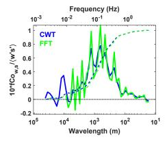
**Figure 5.** Global cospectra of vertical wind and potential temperature for the leg described in Fig. 4, calculated by time-averaging the local wavelet cospectrum (blue) and fast Fourier transforms (green). Cospectra are scaled for display. Dashed lines show the cumulative integrals of the cospectra (ogives), normalized by total covariance.
