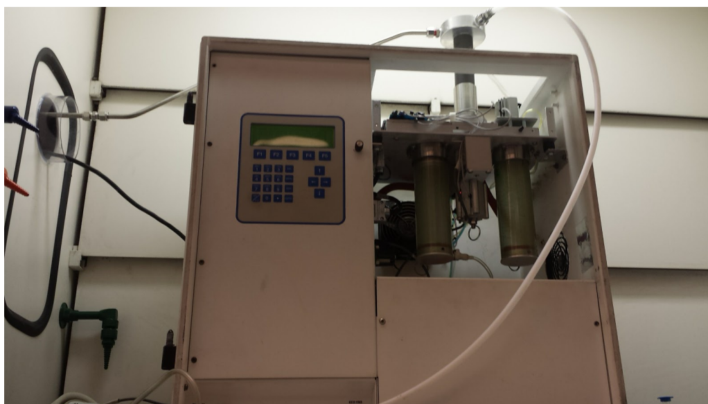
Figure S-2. Partisol Plus 2025 instrument, showing two clear filter magazines within the hollow section of the sampler.
