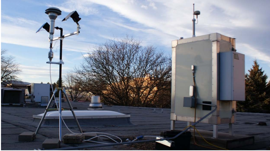
Figure S4: Two AMOD samplers mounted with an FEM gravimetric filter sample and next to the GRIMM FEM monitor for a co-location test.
