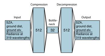
**Figure 10.** Auto-associative neural network used for novelty detection. The input and output layer consist of SZA, ground distance, ground elevation and radiances at 319 wavelengths. The network has three hidden layers with 512, 32 and 512 neurons per layer.
