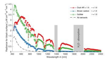
**Figure 2.** Radiance for a black surface, three different aerosol types and no aerosols from an observed altitude of 3 km with an SZA of 25°. Every aerosol type (dust with an AR of 1.5, carbon and sulfate) is shown for an AOT of 1.0. No data are shown for the wavelengths of two water vapor absorption bands (grey bars).
