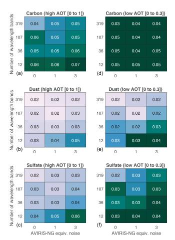
**Figure 7.** Standard error for retrieved AOT of 12 individually trained neural networks with varying wavelength bands (319, 107, 36, 12) and a varying amount of simulated AVIRIS-NG equivalent noise (0, 1, 3; see Eqs. 5 and 6) from the test set. Panels (**a**), (**b**) and (**c**) show the standard error when AOT is varied between 0 and 1. Panels (**d**), (**e**) and (**f**) show the standard error for AOT between 0 and 0.3.
