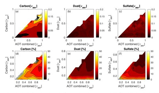
Figure 5. Error in retrieved AOT for carbon, dust and sulfate aerosols on the test set. Panels (a), (b) and (c) show the absolute error, while (d), (e) and (f) show the error in percent. The color mapping is held constant for each row and varies across the three columns.
