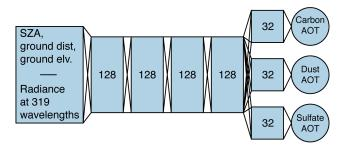
**Figure 3.** Model architecture of the neural network for aerosol retrieval. The inputs consist of the SZA, ground distance, ground elevation and the radiance at 319 individual wavelengths. The network has five hidden layers with 128 neurons in the first four layers and 96 neurons in the last hidden layer. The outputs of the network are the AOT for carbon, dust and sulfate aerosols.
