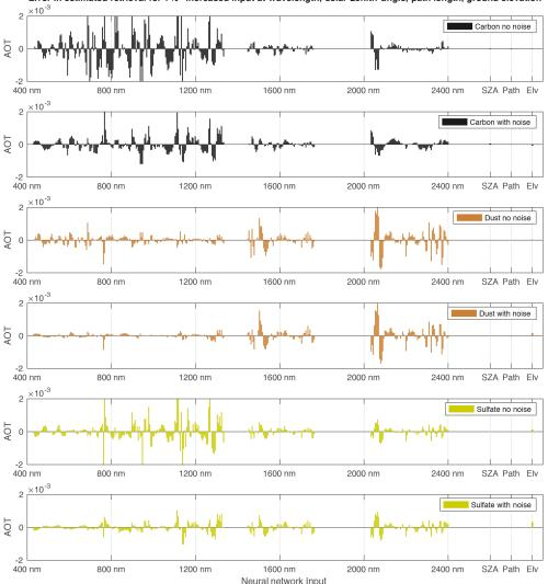
Error in estimated retrieval for 1%<sup>\*</sup> increased input at wavelength, solar zenith angle, path length, ground elevation
