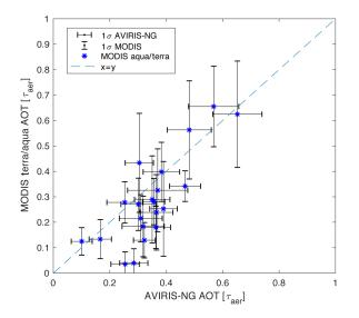
**Figure 16.** AOT retrieved by MODIS (y axis) vs. AOT retrieved by AVIRIS-NG with the model (x axis). The standard deviation for MODIS is shown with vertical bars and the standard deviation for the retrieval with horizontal bars.
