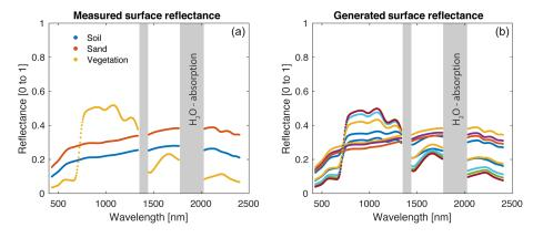
Figure 1. (a) Surface reflectance for three different surface types (soil, sand and vegetation) from measured and smoothed surface spectra. (b) Nine surface spectra randomly generated from the three spectra on the left. Wavelengths with strong water vapor absorption are marked in grey.
