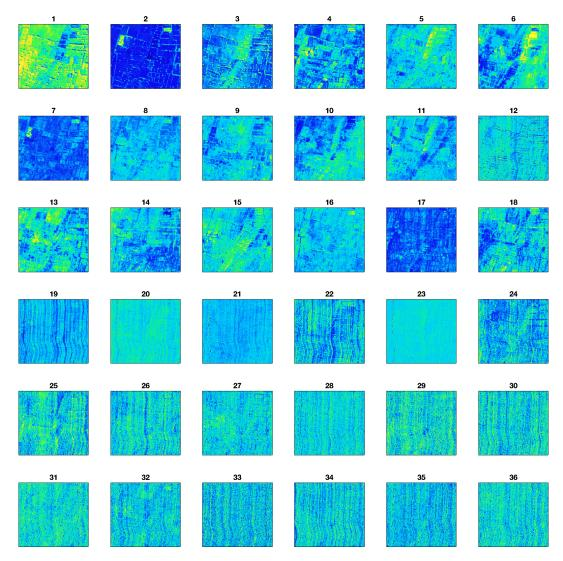
**Figure 9.** First 36 eigen-images from an AVIRIS-NG flight on 10 January 2016 near Coimbatore, India. Shown is a spatially resolved scene of  $100 \times 100$  ground pixels, approximately  $500 \times 500$  m. Instrument artifacts (vertical stripes) are visible for eigen-images numbered higher than 16 (for example, 19 and 22).
