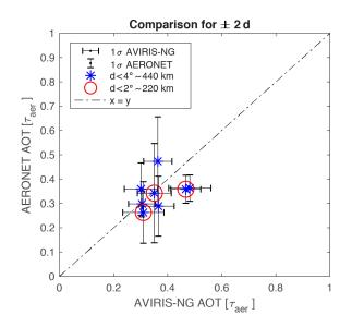
**Figure 15.** AOT retrieved by AERONET (see Eq. 12) and the AOT retrieved from AVIRIS-NG with the model. The standard deviation for AERONET is shown with vertical bars and the standard deviation for the retrieval with horizontal bars. All comparisons between AERONET and AVIRIS-NG flights are located within  $4^{\circ}$  ( $\approx 440 \text{ km}$ ) and within 2 d of each other. The three comparisons within  $2^{\circ}$  ( $\approx 220 \text{ km}$ ) are circled in red.
