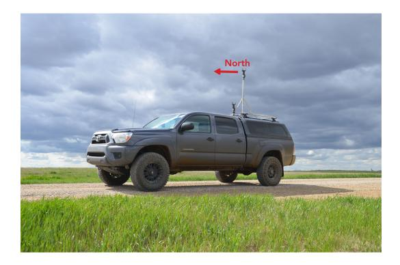
Figure S1: Field photo showing the location of both anemometer placements. The North arrow indicates that the anemometers were positioned with the  $0^{\circ}$  reference was in line with the front of the truck.
