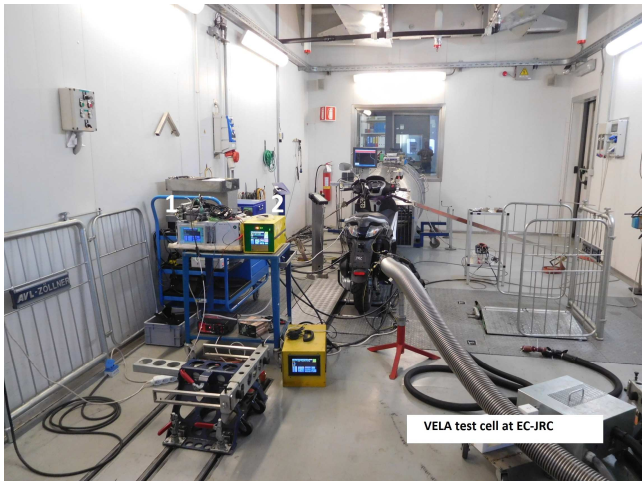
Picture S3: Example of validation test for Mini-PEMS No.1 and No. 2. Mini-PEMS No. 1 was installed on-board of the vehicle during emission roller bench tests.
