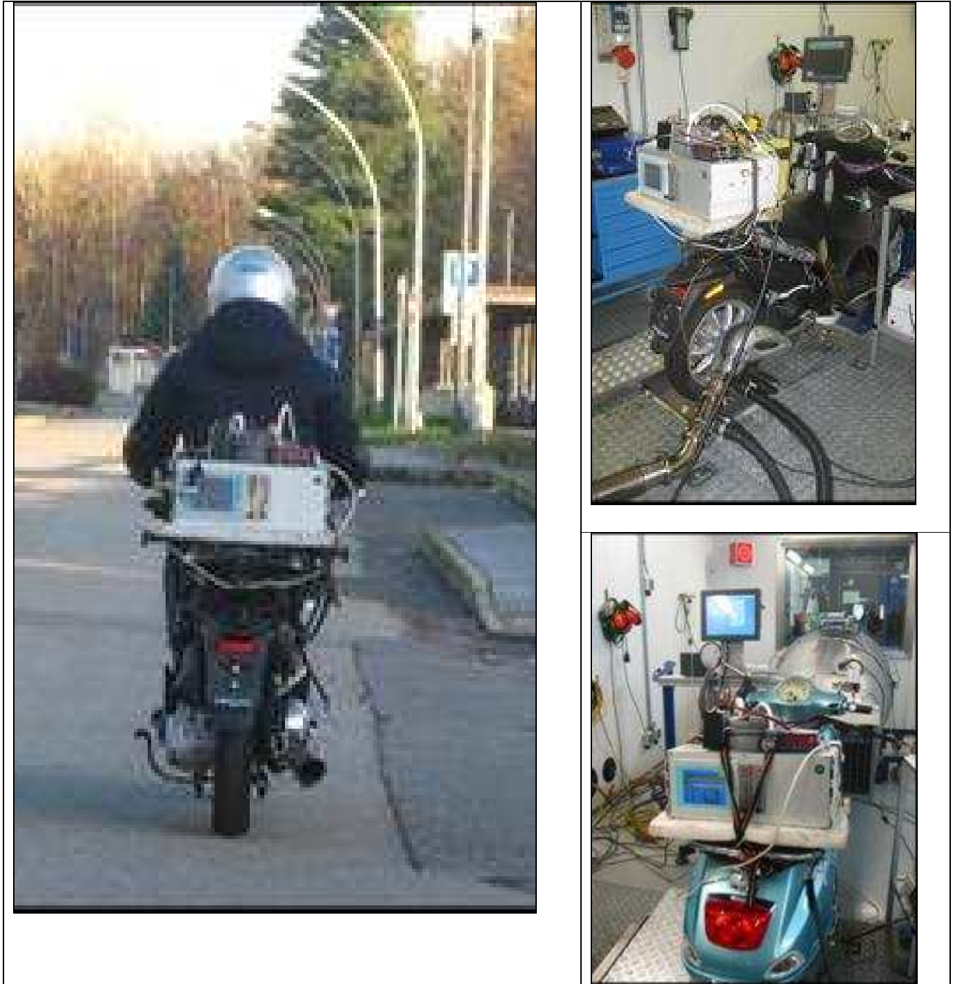
Picture S1. Example of Mini-PEMS No. 1 installed on 2-wheelers during tests on the road (left) and during roller bench tests (right).
