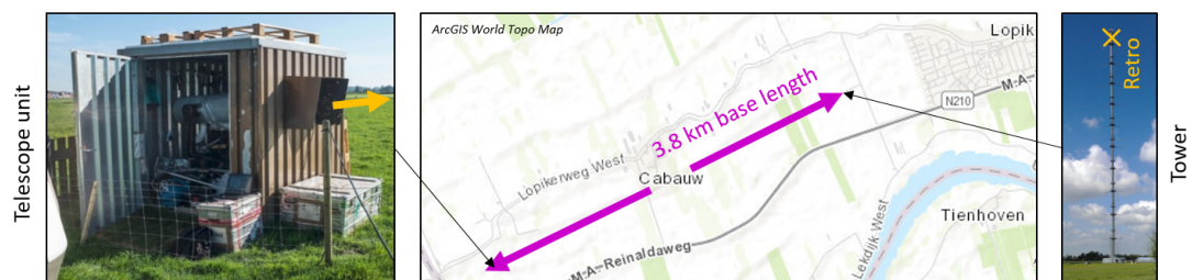
Figure S8. Setup of the LP-DOAS system. As shown on the map (Esri et al., 2018), the light sending and receiving telescope unit (left) was located at 3.8 km distance to the meteorological tower (right), resulting in a total light path of 7.6 km. There were several retroreflectors installed on the tower at different altitudes. However for this study, only the one at the very top (207 m altitude) was used to obtain the average gas in the lowest retrieval layer, extending from 0 to 200 m altitude.
