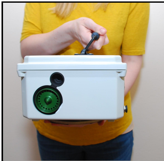
Image: How to hold the AMOD sampler.
