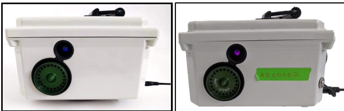
Image: When charging, AMOD LED light will be blue (left) or pink (right).
