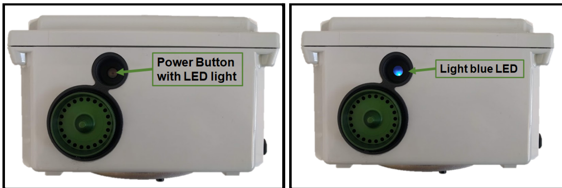
Image: CEAMS sampler showing the power button before (left) and after (right) it is pressed and paired with a mobile phone.
