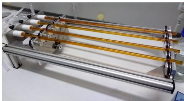
65 Figure S3: Created system (called “Denudermaster”) for the simultaneous coating of four denuders.
