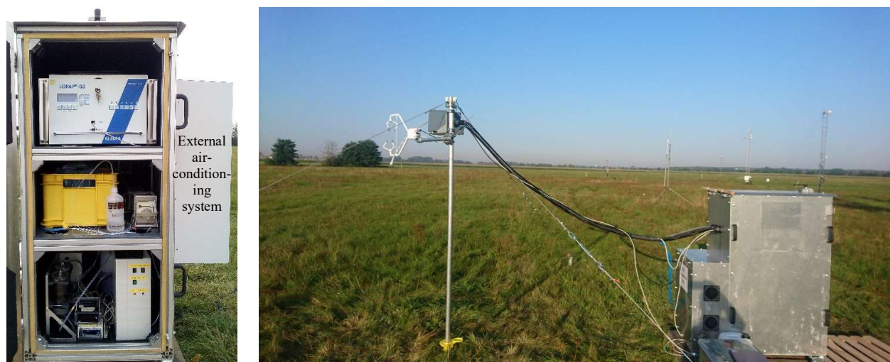
Figure S5: Left: opened field rack with LOPAP (upper level), reagents and external peristaltic pump (middle level), electronics and zero-generator (lower level) and external air conditioning system (side); right: field rack with mast for the external sampling unit and the anemometer.
