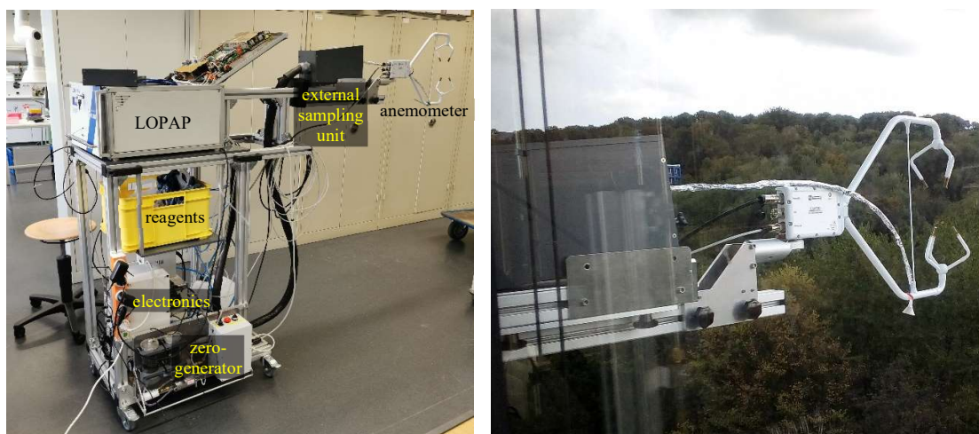
Figure S4: Laboratory set-up: left: moveable laboratory rack; right: external sampling unit and anemometer in the atmosphere in front of the facade of the laboratory.
