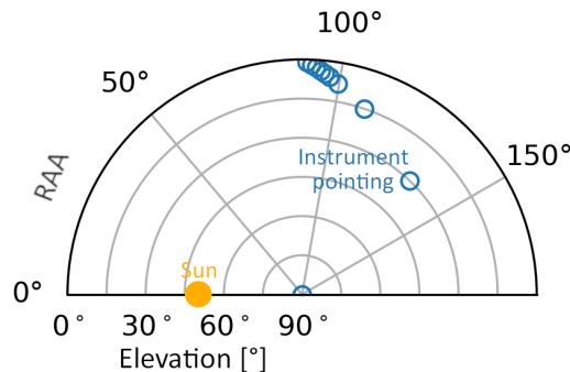
**Figure S5.** Viewing directions for a tilted elevation scan. For a given EA sequence and SZA, the RAA is chosen to realise a single scattering angle as close to  $90^\circ$  as possible. In this example the EA sequence according to Table 3 in the main text and an SZA of  $40^\circ$  was assumed.
