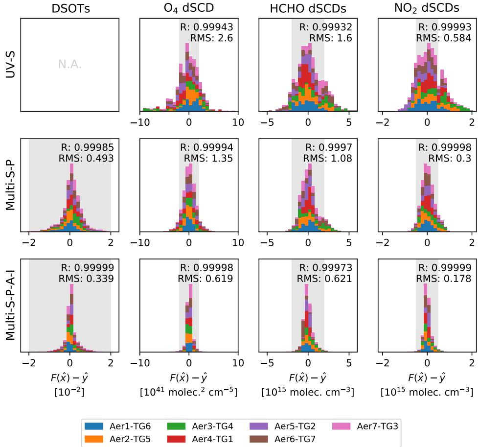
**Figure S11.** Deviations between the input observations  $\hat{y}$  and the modelled observations  $F(\hat{x})$  for the retrieved states  $\hat{x}$ , illustrating the quality of the convergence. Sub-plot columns show different kinds of observations. Sub-plot rows represent different measurement modes. Y-axes are occurrences in arbitrary units. Grey-shaded areas indicate the assumed measurement uncertainties according to Table 1. RMS values are given in the horizontal axes' units.
