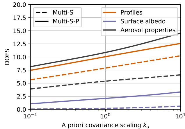
**Figure S15.** Investigation on the impact of the choice of  $\mathbf{S}_a$  on the DOFS reported in this study. The figure shows the behaviour of the DOFS for various measurement modes and parameter subgroups, when  $\mathbf{S}_a$  is scaled by a factor  $k_a$ . Calculations were performed for  $\theta = 60^\circ$ ,  $\phi = 90^\circ$ , and Aer1-TG1 profiles.
