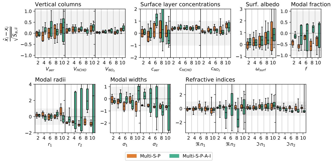
**Figure S14.** Statistical representation of the retrieval results for the Multi-S-P and the Multi-S-P-A-I modes, with inhomogeneity noises of different magnitudes. The x-axes of each subplot indicates the noise magnitude in percent. The figure is organised in a similar manner to Figure 11 in the main text.
