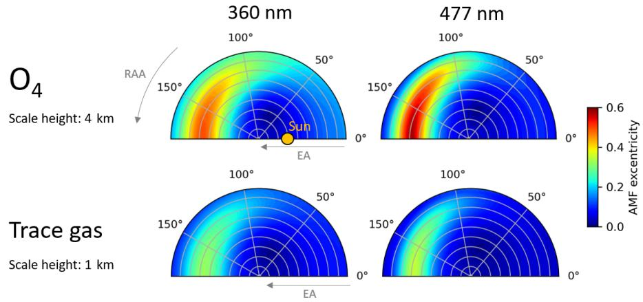
**Figure S1.** Eccentricity of the AMF modelled over the sky hemisphere for a Rayleigh atmosphere in two major  $O_4$  absorption bands at 360 and 477 nm, respectively. The upper row shows AMFs for  $O_4$ , while the bottom plots show AMFs for an arbitrary trace gas confined to lower altitudes (exponential profile with scale height of 1 km).
