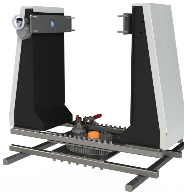
Figure 3. The alt-azimuth positioner with its two side arms and the base.
