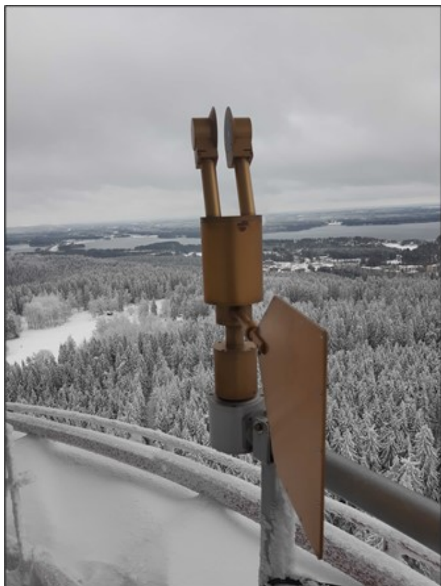
Figure 1. ICOMET sensor located in Puijo tower. The height of the ICOMET sensor is 53 cm and the weight is 8 kg. The wind wing is used to align the sensor according to the wind direction. (Photo credit: Ari Leskinen).
