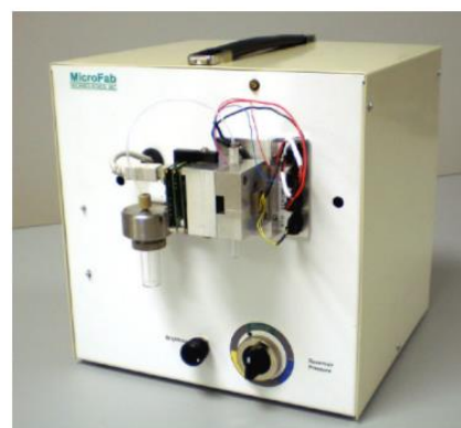
Figure S9. Vaporjet from MicroFab Technologies. (a) View of the microjet dispenser where the droplets are dispensed and evaporated by the white heater. (b) The whole instrument is equipped with different pressure regulators and a stroboscopic camera (VaporJet, MicroFabTechnologies).
