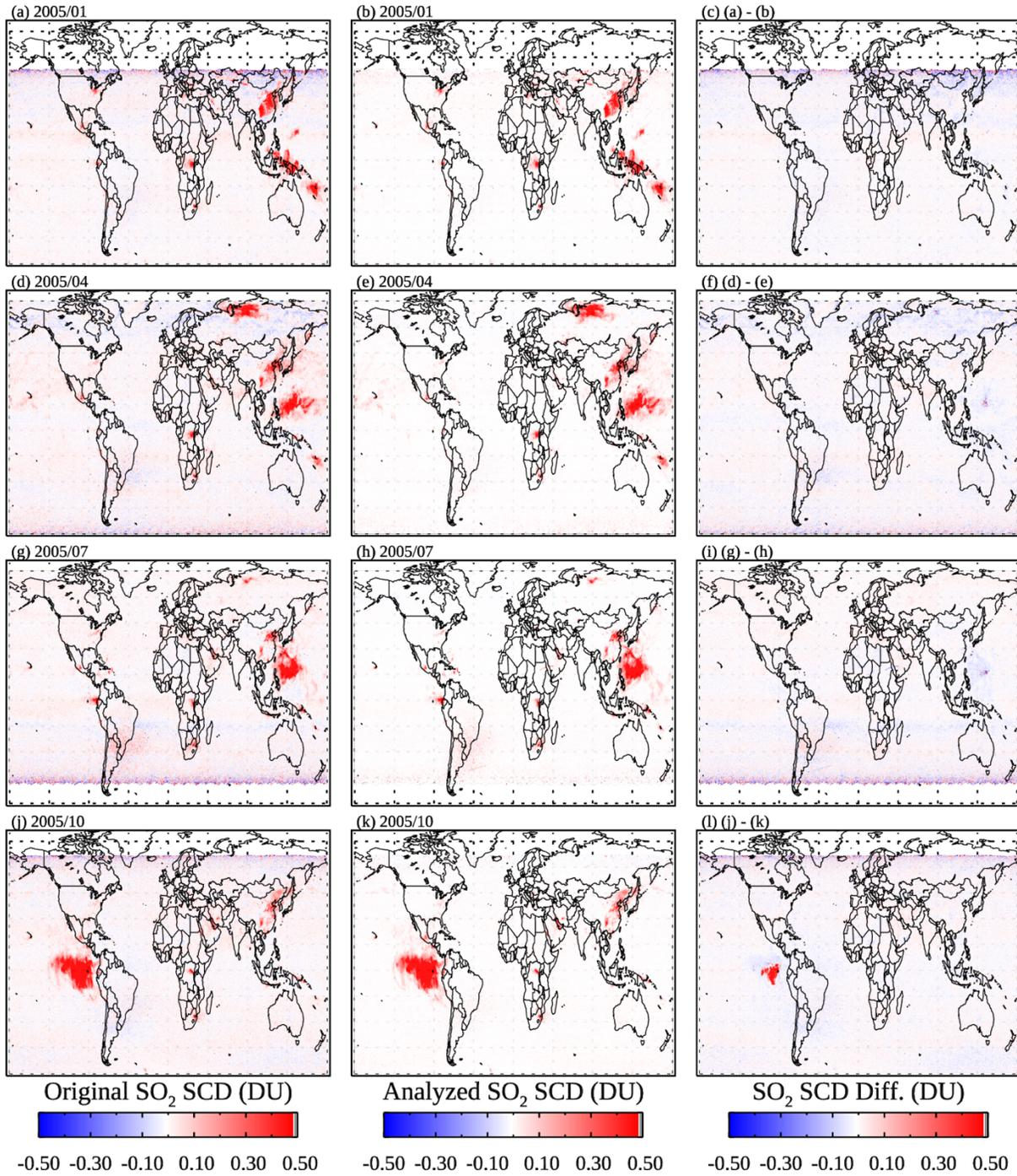
Figure S2: Monthly mean SO<sub>2</sub> SCDs for March 2005 from (first column) the original PCA retrievals and (second column) the neural network based analysis, and (third column) their differences for (a-c) January, (d-f) April, (g-i) July and (j-l) October 2005.
