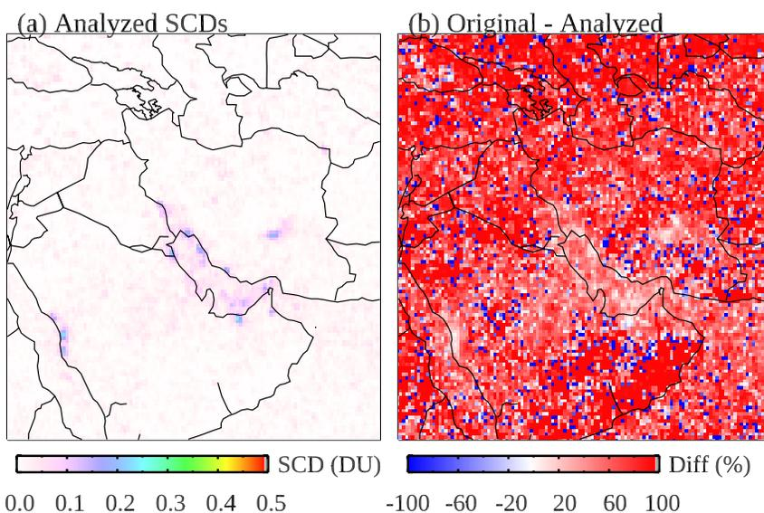
**Figure S4:** Same as Figure 6 but for the Middle East. For polluted areas ( $SCD_{NN} > 0.15$  DU), the mean relative difference between the original and analyzed SO<sub>2</sub> SCDs is 14%, with the original being greater.
