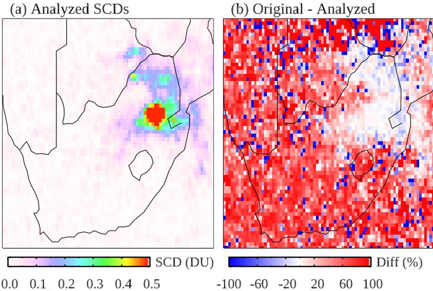
**Figure S5:** Same as Figure 6 but for South Africa. For polluted areas ( $SCD_{NN} > 0.15$  DU), the mean relative difference between the original and analyzed  $SO_2$  SCDs is -1%, with the original being smaller.
