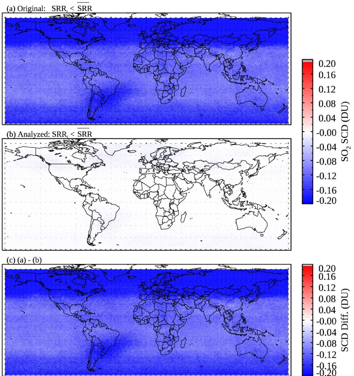
Figure S9. The (a) original, (b) NN analysed OMI SO<sub>2</sub> SCDs and (c) their differences for March 2005 for pixels with SCD/RMS ratios ( $SRR_i$ )  $< \overline{SRR}$ , where  $\overline{SRR}$  represents the monthly median of the daily mean SRRs calculated for each 3° latitude band.
