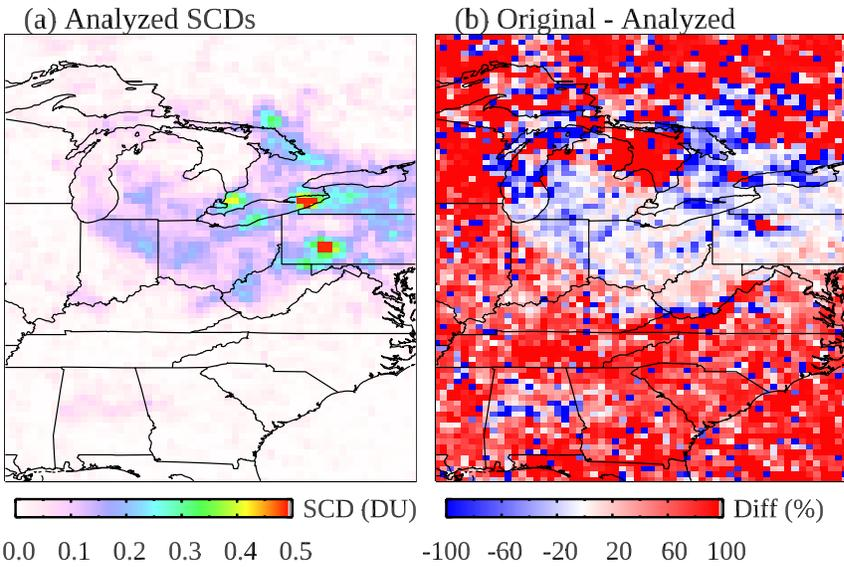
**Figure S6:** Same as Figure 6 but for the eastern U.S. For polluted areas ( $SCD_{NN} > 0.15$  DU), the mean relative difference between the original and analyzed  $SO_2$  SCDs is -11%, with the original being smaller.
