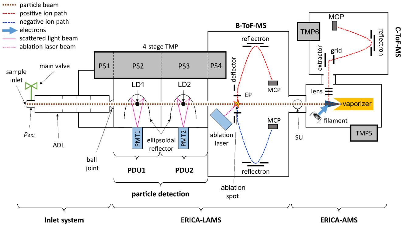
Figure S1 - A simplified drawing of the ERICA mass spectrometer. This figure is also presented in Hünig et al. (2022).
