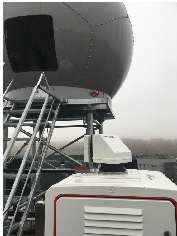
Figure 1. Vaisala WRS400 X-band radar and WindCube 400S Doppler lidar installed on the roof of a building at Vaisala Oyj headquarters in Vantaa, Finland. Photo credit: Raisa Lehtinen.
