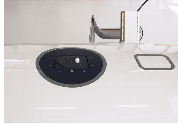
Figure S7. Photograph of the HALO top fuselage with instrument apertures. Left: Instrument plate installed in a larger, black adapter flange for the FLV configuration. Right: standard aperture used for FLT and FLN configurations (closed with a white blind flange).
