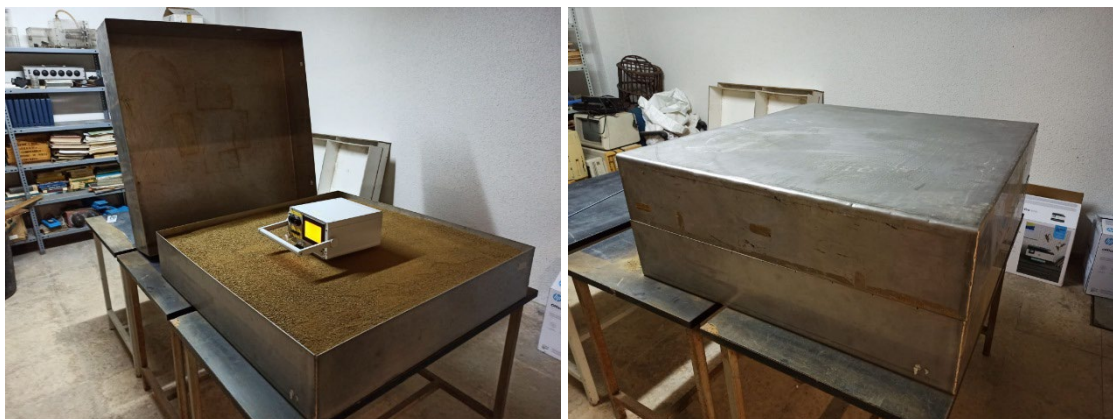
Figure S1. Picture of the setup used to empirically determine the exhalation rate reference value of the EB.
