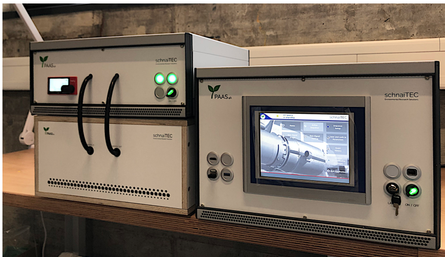
Figure S1. Photograph of the PAAS-4λ consisting of the Optics Unit (lower left ), the Flow Unit (upper left), and the Electronics Unit (right).
