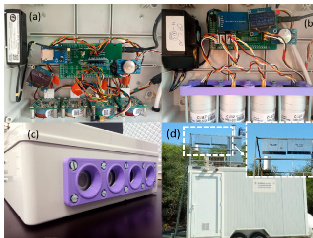
Figure 1. Images showing the layout of the AQ monitors housing the Alphasense (a) and the Winsen (b) LCSs, the side of the AQ monitors at which the sensing elements of the LCSs were exposed to the ambient air (c), and the place that the AQ monitors were installed at the top of the reference station (d).
