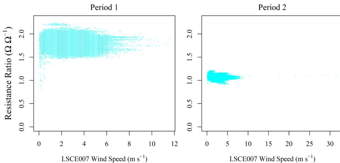
**Figure S5:** The ratio between measured Figaro resistance and standard 2 ppm [CH<sub>4</sub>] reference resistance (cyan dots) from the SUEZ Amailloux landfill site for LSCE007, plotted against minute-averaged wind speed as measured by the LSCE007 anemometer, for wind directions between 180° and 270°. Data from period 1 is plotted on the left and data from period 2 is plotted on the right.
