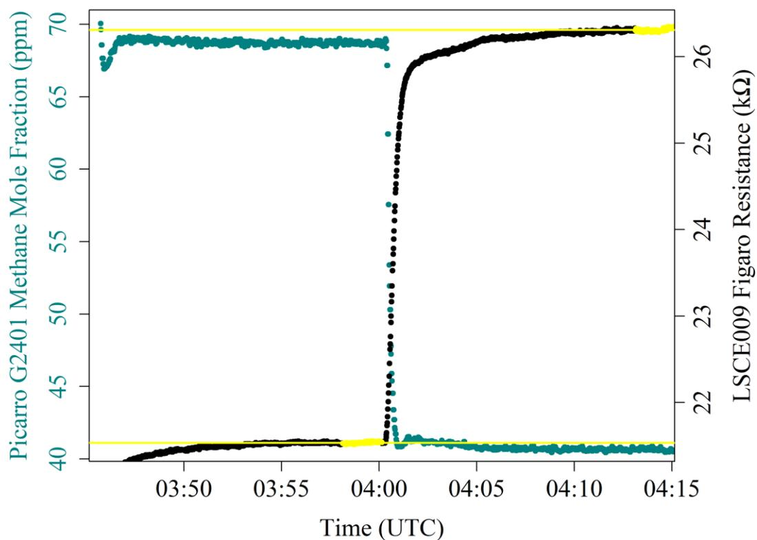
Figure S3: A methane mole fraction transition from 69 ppm to 41 ppm as recorded by the Picarro G2401 (dark cyan dots on left-hand axis) with corresponding LSCE009 Figaro resistance measurements made in System B (black dots on right-hand axis). 2 minutes of stable Figaro resistance sampling from the end of each sampling period (highlighted yellow dots) were used to derive resistance averages (horizontal yellow lines).
