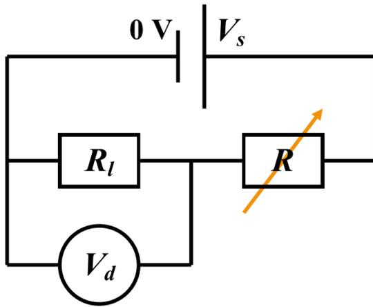
Figure S2: Circuitry used to measure the resistance of the Figaro sensing element. See text in Sect. 2.1 for labels.
