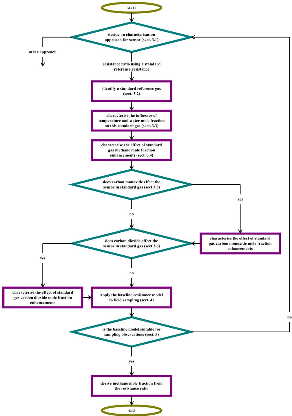
Figure S1: A flow chart illustrating the various steps that we followed in order to derive methane mole fraction from the Figaro TGS 2611-E00.
