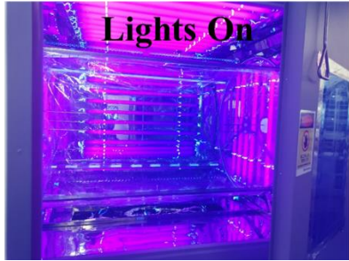
Figure S1. Pictures of this AIR Teflon chamber (reactor and its enclosure)
