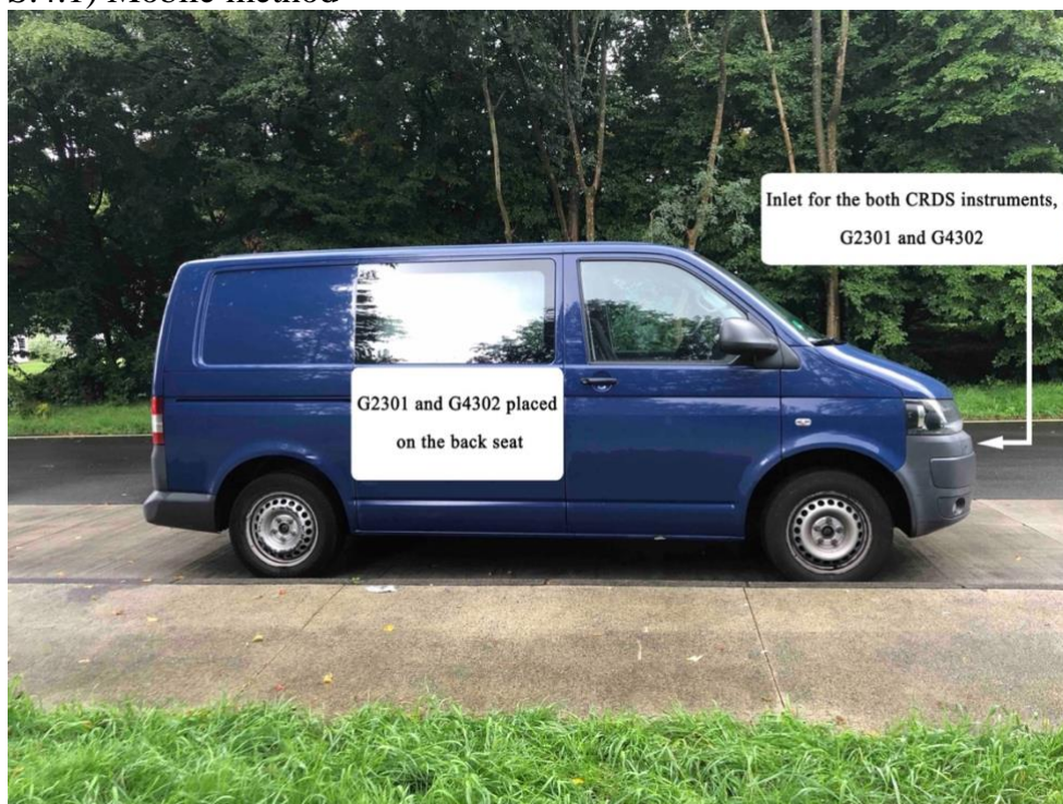
Figure S4 - Mobile measurements vehicle
