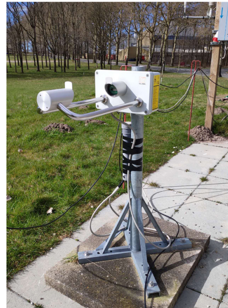
Figure 5. The Thies laser precipitation monitor (LPM) at DTU Risø campus.
