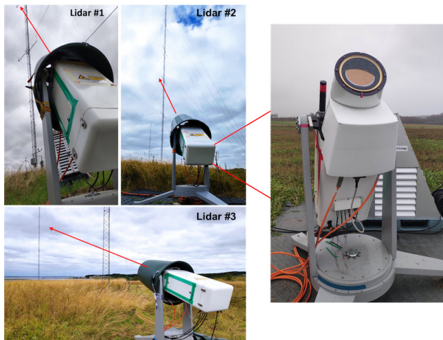
Figure 1. The three CW lidars were pointed at a common focus point close to a sonic anemometer on a met mast at DTU Risø campus.
