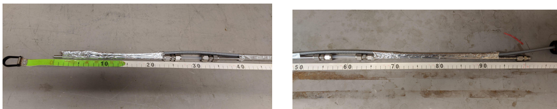
Figure S9. The head (left panel) and base (right panel) sections of the interior tubing of the profiling arm, including two 5 cm PTFE lengths.
