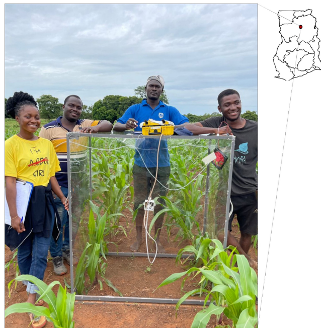
Figure 4. Transparent (NEE) manually operated closed-chamber measurement at the CSIR-SARI experimental field, used for field trial application of the developed low-cost CO 2 and ET flux measurement device, near the city of Nyankpala, northern Ghana (9°24′15.9″ N, 01°00′12.1″ W).
