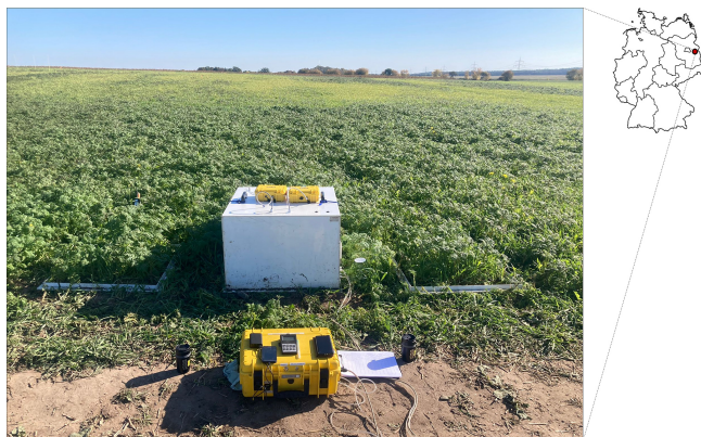
Figure 3. Parallel opaque ( R_{\text{eco}} ) manually operated closed-chamber measurements with a LI-COR 850 IRGA (LI-850, LI-COR, USA) and the developed low-cost CO 2 and ET flux measurement device at ZALF experimental field near the village of Tempelberg, northeast Germany (52°26′49.2″ N, 14°09′00.0″ E). The developed system was equipped with a K30 FR and SCD30 NDIR, as well as SHT31 and DHT22 sensors.
