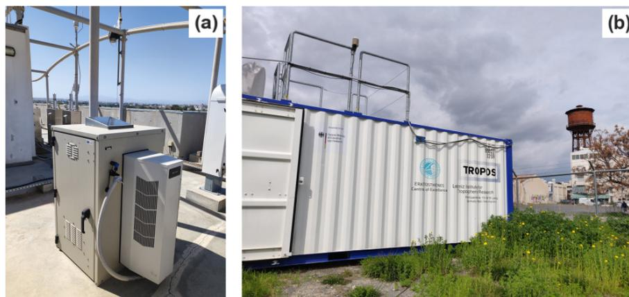
**Figure 1.** CE376 lidar with thermal enclosure on the roof of the premises of The Cyprus Institute in Nicosia (a) and Polly<sup>XT</sup> container housing at CUT premises in Limassol (b).
