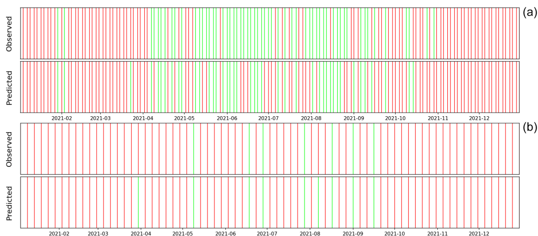
Figure 4. Time series of predictions for sites T 7 (a) and T 17 (b) over the test year (2021). Green (red) lines indicate that a plume was (was not) observed or predicted. Observed ground truth values are shown in the upper time series and CH4Net predictions in the lower time series. The date format is year-month.
