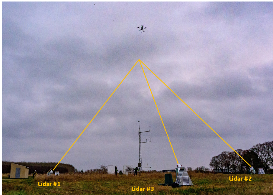
Figure 3. Experiment setup of the three CW Doppler lidars at the Technical University of Denmark (DTU) Risø campus. The surrounding terrain is relatively flat and agricultural. The three lidars focus at about 8 m above the top of a met mast.
