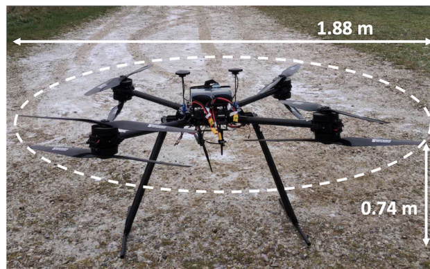
Figure 1. The Foxtech D130 X8 rotary-wing drone used in the experiment.
