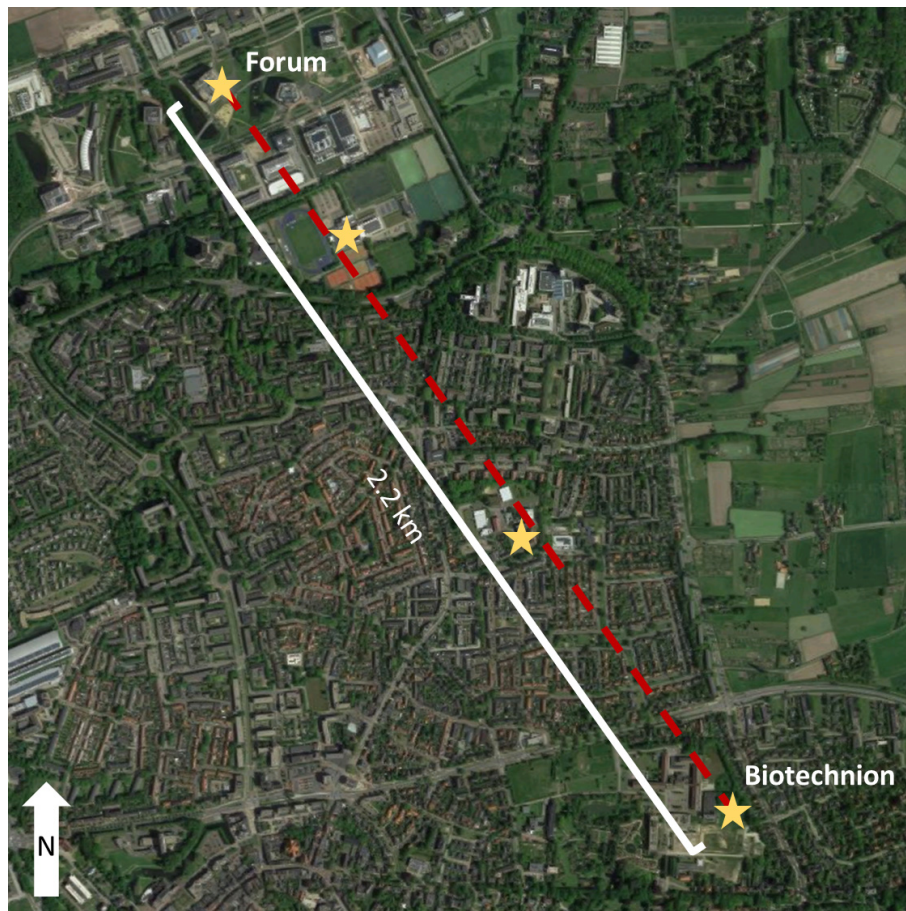
Figure 1. Map of Wageningen, with the path of the links in red. The receiving antennas are at the end labelled “Forum”; the transmitting antennas are positioned at the end labelled “Biotechnion”. The yellow stars indicate the position of disdrometers along the path. At each disdrometer location, one disdrometer is located, except at Forum, which has two disdrometers placed next to each other. Figure redrawn after van Leth et al. (2018a) (© Google Maps).
