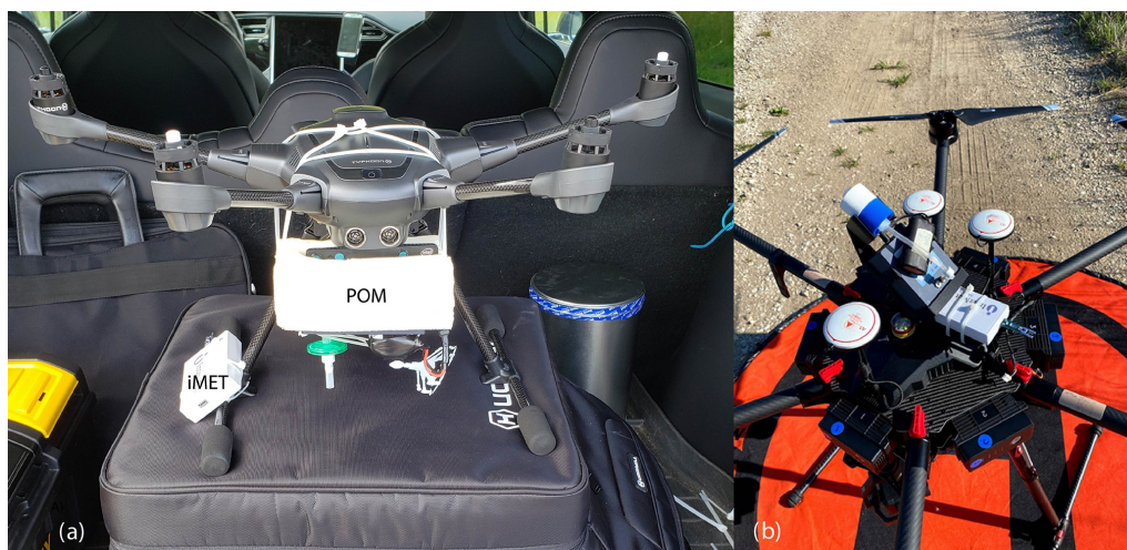
Figure 2. (a) Typhoon H UAS with mounted POM and iMet-XQ2 as flown during CHEESEHEAD19 in 2019. The POM was housed in foam for vibration dampening. (b) A top-mounted iMet-XQ2 and POM on a DJI M600 as flown in September 2020 for WiscoDISCO20. The inlet to the POM is held up with a bracket to hold the inlet filter assembly (blue and white).
