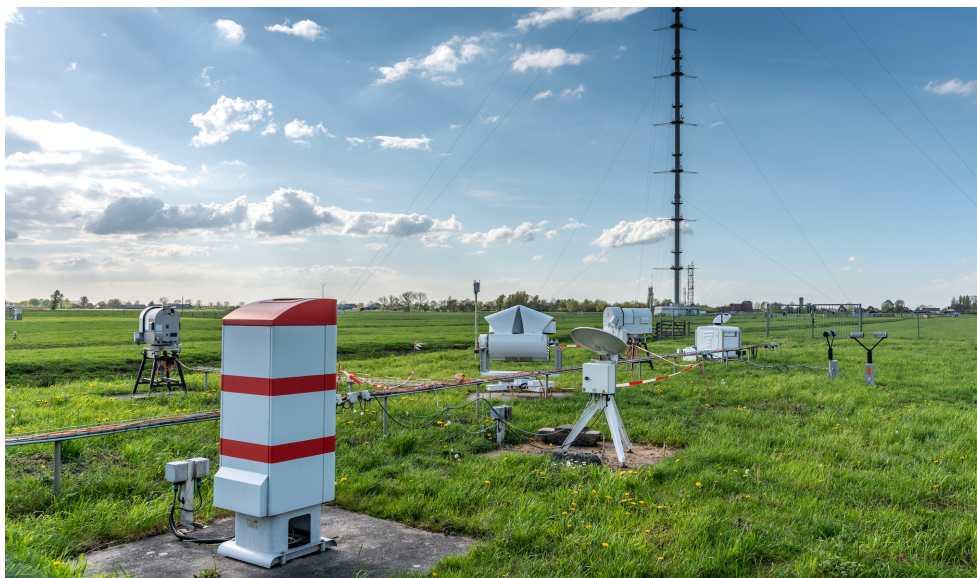
Figure 2. The ceilometer (in front) and 213 m mast (background) at the same location at Cabauw support high-quality annotations. This site also includes a scanning microwave radiometer (left); a scanning cloud radar, a micro rain radar, and a second microwave radiometer (centre); and a scanning Doppler wind lidar and two distrometers (right).
