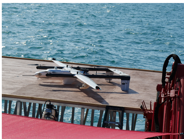
Figure 5. FVR-55 with the clear-sky payload on board on the 6\text{ m} \times 6\text{ m} launch pad on the rear deck of the TowBoatU.S. Richard L. Becker .
