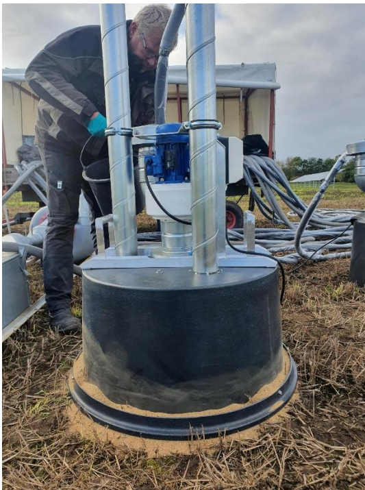
Figure S4. Dynamic flux chamber in the field with sand sealing at the soil surface.
