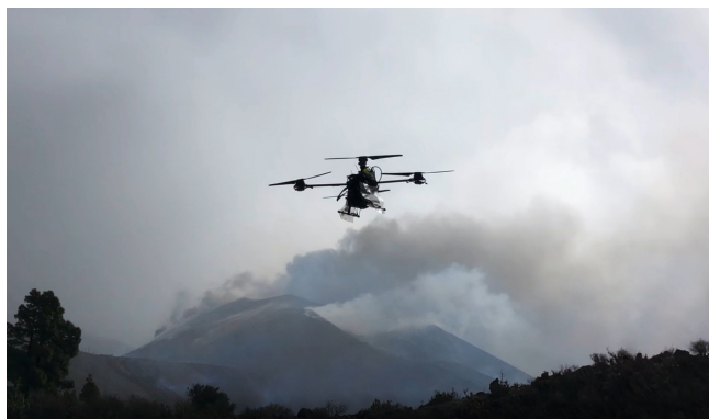
Figure 1. A Dragonfly UAS returning from a CO 2 sample mission during the November 2021 eruption of Tajogaite volcano. The large volcanic ash plume is visible in the background and contains an invisible CO 2 plume, which was the mapping target of this drone.
