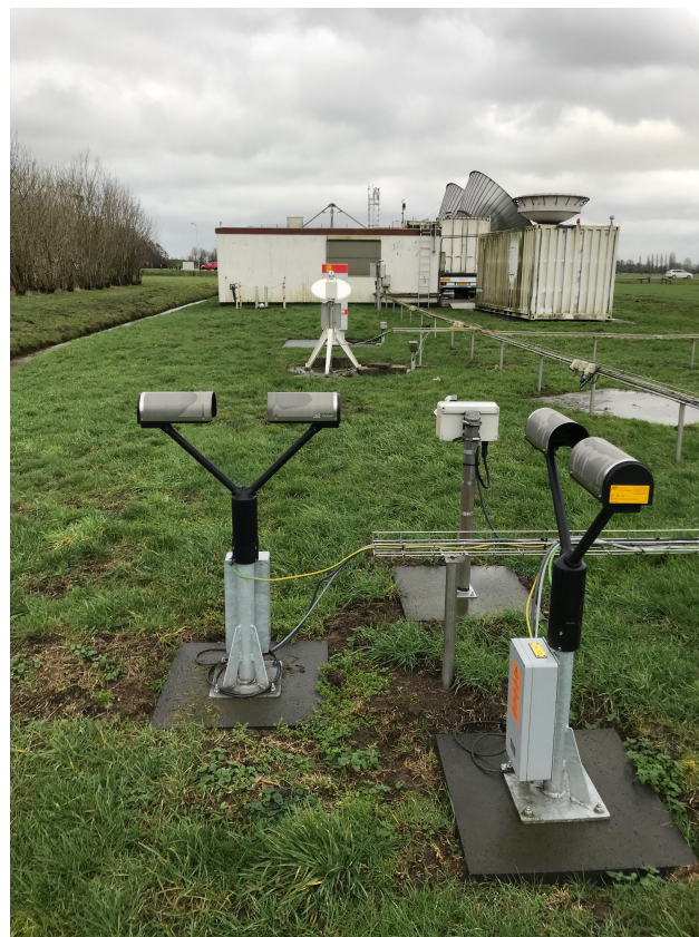
Figure 1. Parsivel 2 disdrometers at the Cabauw Experimental Site for Atmospheric Research in the Netherlands. The micro-rain radar is visible in the background.
