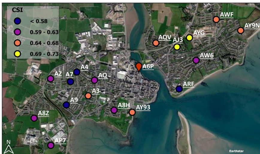
Figure 9. Dungarvan AQStations locations with CSI results indicated in coloured circles (blue is the lowest CSI; yellow is the highest CSI) and the A6P location indicated by red pin marker. (map obtained from Esri, DigitalGlobe, GeoEye, i-cubed, USDA FSA, USGS, AEX, Getmapping, Aerogrid, IGN, IGP, swisstopo, and the GIS User Community).
