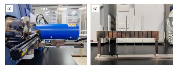
**Figure S1** (a) DART-MS/MS set up during analysis. (b) Metal holder with six glass capillary tubes on a stainless steel stand. The center-to-center distance between two glass capillary tubes is 18 mm.
