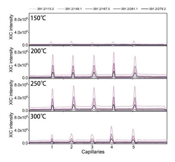
**Figure S2** Temperature variations of the extracted ion chromatograms (XIC) obtained from 5 capillaries samples for spiked DEHP within 4 minutes. The He flux temperature was set at 150 °C, 200 °C, 250 °C, and 300 °C due to the boiling points of DEHP were 384 °C.
