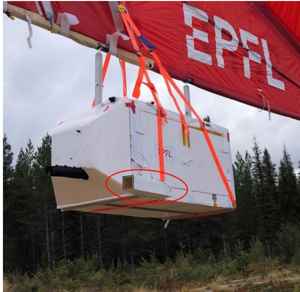
10 Figure S1: MoMuCAMS with the additional radiation shielding for temperature sensors installed on the side (in the red ellipse). The tube shaped radiation shield includes a net on the front to prevent condensation of water directly on the sensors and a fan in the back to provide active flow of air through the tube. Two T and RH sensors (SHT85, Sensirion, CH) are placed in the middle of the tube.
