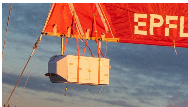
Figure 1. Picture of the MoMuCAMS payload attached to the Helikite. Two aluminum bars connected directly to the Helikite's structure ensure stability of the payload. Two additional cargo straps provide additional safety for the payload attachment. The system remains very stable, even at winds above 15 \text{ m s}^{-1} .
