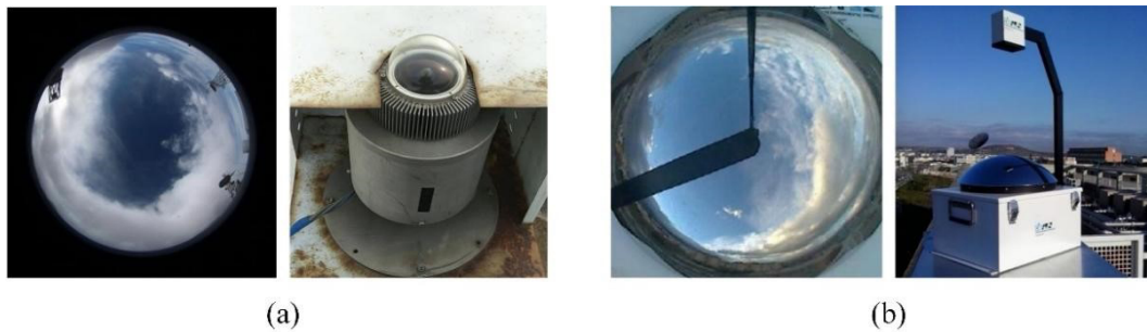
Figure 1. Two kinds of ground-based cloud images and their observation equipment: (a) ASI ground-based cloud image and its observation equipment (Cazorla et al., 2008; Shi et al., 2019); (b) TSI ground-based cloud image and its observation equipment (Long et al., 2006).
