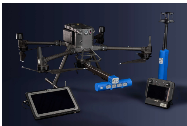
Figure A3. Methane sensor showing location of integrated GPS and lidar attached to the quadcopter drone.
