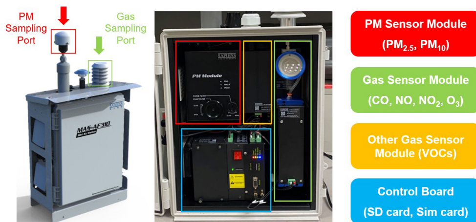
Figure 1. Structure diagram of a MAS monitoring device (dimensions: 420 \times 320 \times 180 mm, H \times W \times D ; weight: 12 kg; power consumption: 15 W).
