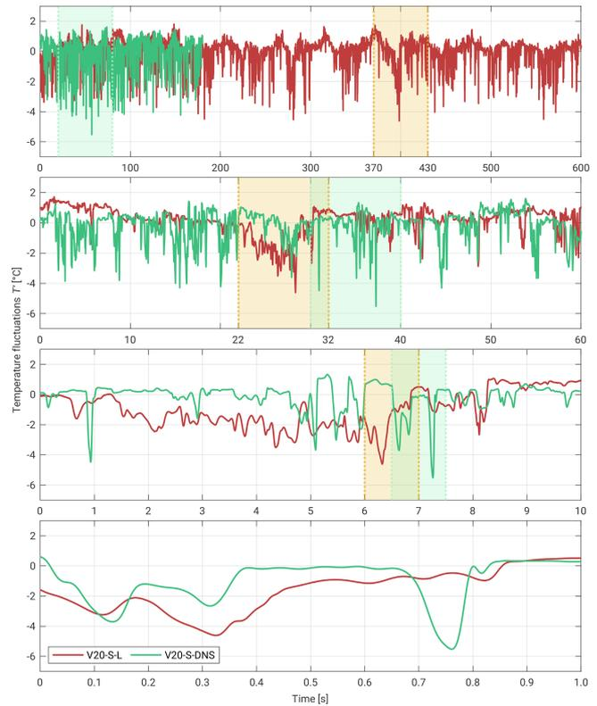
**Figure A2.** Experimental versus DNS  $T'$  series  $\sim 5$  cm below the ceiling shown in the following zoomed-in time segments: 600, 60, 10, and 1 s. The presented dataset covers the  $\Delta T = 20$  K case. Please note that the time series from the experiment and the DNS do not correspond to each other.
