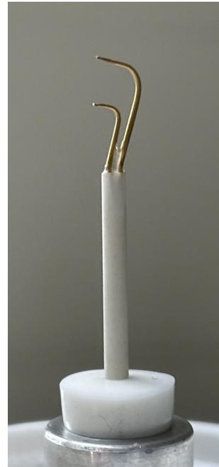
**Figure 1.** UFT-2B head sensor. Parallel to the mean flow, tungsten wire (2.5  $\mu\text{m}$  thick, 3 mm long) spanned a miniature industry standard wire probe by DANTEC<sup>®</sup>.
